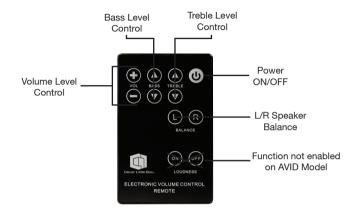
Using the supplied IR Remote Control will give access to further features and functions of the AVID and will allow adjustments to the sound levels and tone settings.
