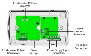
Screw terminal connections for Power, Wired Input Loudspeaker Outputs and Line Level outputs are located on the rear PCB of the AVID.
