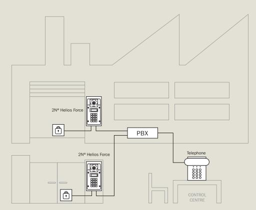
Industrial operations are usually equipped with an exchange, and the environment is analogue. In such a case the analogue 2N<sup>®</sup> Helios Force is suitable for securing entries and exits. At the gate it can withstand the attacks of vandals, dust and water. It can be connected with the control centre of the security service or camera system.
