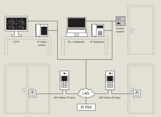
In an office environment it is possible to connect 2N® Helios IP Vario with any IP equipment. In this way it can function as part of the attendance system or CCTV system. The video from the intercom can be displayed very easily on an IP video telephone, notebook or tablet. You can easily integrate the intercom into the existing IP infrastructure.
